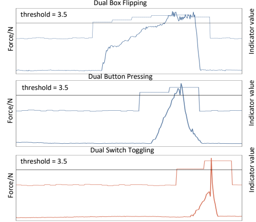
Fig. 9. Multimodality indicator value and force curves on the three contact-rich tasks. The indicator value remains lower before contact and during target approach, then rises with the force response in contact-rich phases, supporting the switch from the low-frequency sampler to the high-frequency distilled sampler.
